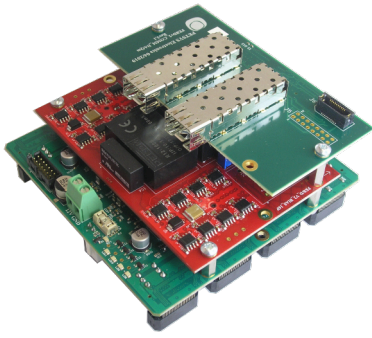
Figure 6: FEB/D-1k module. Top view of the FEB/D-1k module showing the bias voltage mezzanine (red) and the SFP+ communication mezzanine (green) on top of it..
